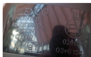
The Milenco mirror here has been approved in the UK (E11) and has an approval number of 03*6154
