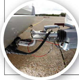
FIG 3 Where no designated attachment point has been provided on the towbar, the cable may be looped around the neck of the towball. Use a single loop only
