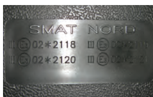
In this example the mirror has been approved in Italy (E3) and has the approval numbers 02*2118 to 02*2121
