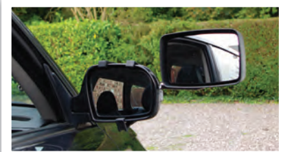
These Reich mirrors can be adjusted from inside the car by pointing a remote control at them
